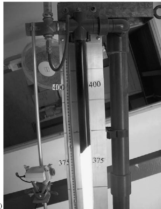
Fig. 3. Visualization of the fluidized bed at vertical and inclined columns: (a) flow of the fluidizing agent through the packed bed of particles, \alpha = 90^\circ , Q = 0.4 l/min; (b) escape of the fluidized bed in an inclined pipe, \alpha = 60^\circ , Q = 7.3 l/min. All particles accumulate at the column's top region.
